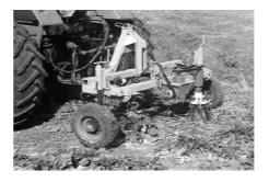
Fig. 1. Scheme of the aggregate: I – integral rowcrop tractor; II–rear-mounted cleaner of the root crop heads: 1 – frame; 2 – linkage system; 3 – tracer wheel; 4 – drive; 5 – cleaning tool
